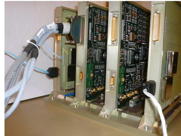
*The new generation of on-board computers based on the LEON3 processor*
